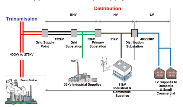
Figure 1 - Typical Electricity Supply Chain
