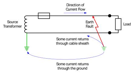
Figure 3 - Earth fault current path
